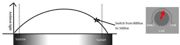
When the LUX Wheel is turned to the mid position this modifies the transition to **night-mode**. Turning the dial towards **EARLY** ensures the transition is made at dusk rather than when the sun has set.
