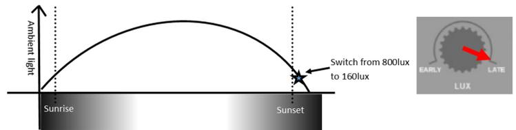
LUX Wheel switched to LATE ensures the light only dims to night-mode when the sun has well and truly set.
