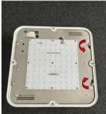
2. Swivel clips to unlock gear tray.
