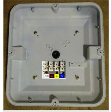
4. Mount base to the ceiling using 5mm x 25mm nail-ins. If IP65 rating is required use cable gland & side entry on the side opposite the LED driver.
