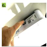
Once aligned, press the light upwards to connect. Do not force the light into the base terminal without aligning the pins and clicking the hinges as the pins may snap. Push barrel lock in to secure.
