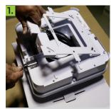
Place the light on a soft surface to avoid scratching the diffuser. Using the key taped to the body of the light, remove the base by turning the key and pulling on the barrel lock.
