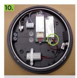
Ensure battery connector is firmly inserted to the driver and write date of commissioning on battery
