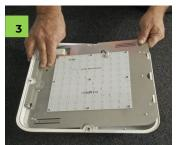
Push gear tray down opposite the swivel clips to take gear tray out.
