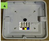
Mount base to the surface. If IP65 rating is required use cable gland & side entry on the side opposite the LED driver and seal screw holes.
