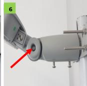
Loosen bolt, adjust tilt angle then tighten. See first page for recommended tilt angles.
