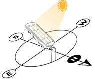
Orientating the solar panel so it faces **North** will ensure optimal charging. East or West facing solar panel can reduce charging of the battery by up to 30% in winter. The solar panel should **not** be facing South. Orientations other than North East, North and North West may void the battery warranty.
