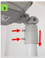
Slip the slip fitter onto the pole. Fits 45-60mm O/D round poles. Ensure solar panel faces North. Tighten bolts to secure to pole. Do not overtighten.
