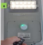
Program fitting with remote control (see page 2 & 3). It may be advantageous to program before mounting the fitting at height.
