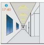
As the light level drops below the threshold, the light goes into standby dimming level.
