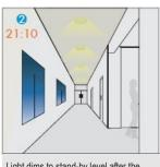
Light dims to stand-by level after the hold-time (no motion).
