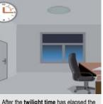
After the **twilight time** has elapsed the light switches to off.
