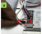
Plug battery connector into driver and note date of commissioning on battery.
