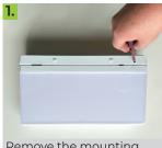
Remove the mounting bracket by inserting a screwdriver into the locking tab
