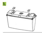
Mount suspension clips to ceiling and attach to WPB
