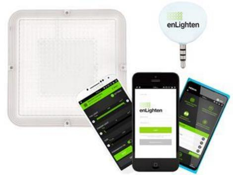
The Chamaeleon™ III is a self-contained LED luminaire available in Standard and Emergency versions. The light operates in 2 modes: Standby Mode and Full Light Mode. When movement is detected in proximity to a Chamaeleon the light operates at full output for a set period of time. The light then slowly fades to Standby Mode. The integrated daylight sensor can be used to keep the light at standby level during daytime.
