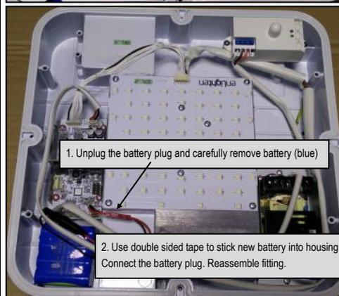
1. Unplug the battery plug and carefully remove battery (blue)
