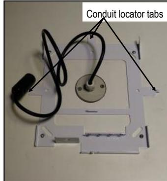
3. Connect the IP65 cable to a suitable water proof junction box. The conduit locator tabs can be used to hold the conduit in the correct position. Standard conduit size is 20mm. For 25mm conduit a reducer is required.
