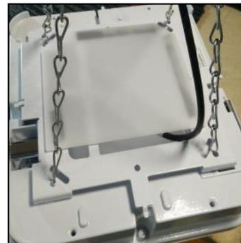
5. Alternatively the fitting can be suspended from the ceiling. Connect the IP65 plug to the fitting then attach the chain to the base plate (as shown above) and wire the mains cable into a junction box.
