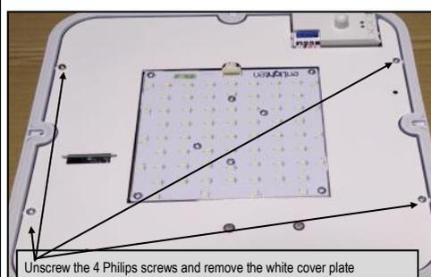
Unscrew the 4 Philips screws and remove the white cover plate
