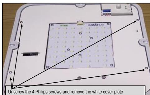
The battery in the IP65 version is located inside the fitting. To replace the battery, remove the diffuser using an Allen key and then remove the white cover plate by unscrewing the 4 Philips screws.
