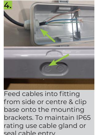
Feed cables into fitting from side or centre & clip base onto the mounting brackets. To maintain IP65 rating use cable gland or seal cable entry.
