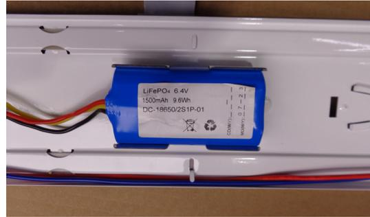
The battery is in a battery holder on the gear tray.
