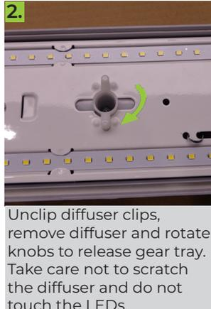
Unclip diffuser clips, remove diffuser and rotate knobs to release gear tray. Take care not to scratch the diffuser and do not touch the LEDs.
