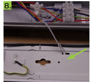
Clip hooks into gear tray to suspend gear tray. The two terminal blocks allow for mains connection in the centre or from the side. Only one of the terminal blocks needs to be connected to power.
