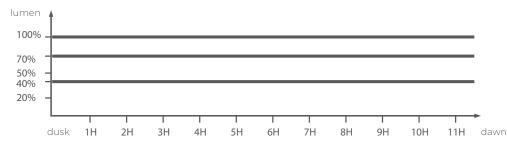
\*Maintaining constant light levels at 100% throughout the night is only possible if the battery is fully charged. Full charging to the battery is unlikely on cloudy days or non summer periods.
