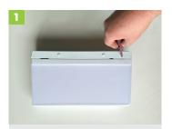
Remove the mounting bracket by inserting a screwdriver into the locking tab.
