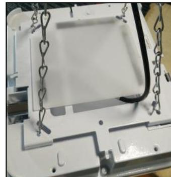
5. Alternatively the fitting can be suspended from the ceiling. A Smart-Connect Base plate with a 3m flex & plug suitable for hanging is available for purchase separately from enLighten Australia. Attach the chain to the base plate (as shown above) and plug the 3pin plug into a power socket or hardwire it into a junction box.
