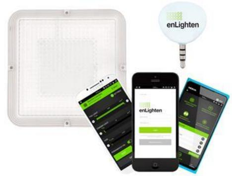
The Chamaeleon™ III is a self-contained LED luminaire available in Standard and Emergency versions. The light operates in 2 modes: Standby Mode and Full Light Mode. When movement is detected in proximity to a Chamaeleon the light operates at full output for a set period of time. The light then slowly fades to Standby Mode. The integrated daylight sensor can be used to keep the light at standby level during daytime.
