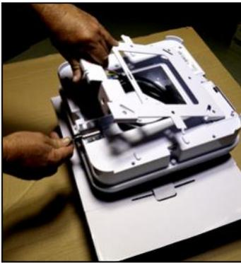
1. Place the light on a soft surface to avoid scratching the diffuser. Using the key taped to the body of the light, remove the base by turning the key and pulling on the barrel lock.
