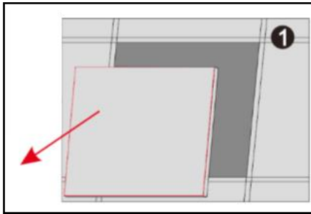
1. Remove ceiling tile
