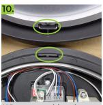
When reattaching the diffuser, align the cutout with the fitting as shown
