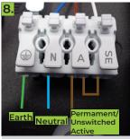
To disable the sensor, bridge terminal A and SE by inserting a cable loop
