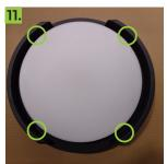
Reattach the diffuser by tighening the 4 bolts holding the diffuser down, ensuring not to overtighten
