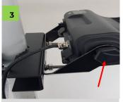
Mount Noctua to angled bracket and tighten the knobs. Connect mains cable to power. Adjust tilt angle as shown above.
